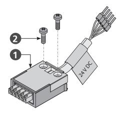
NOTE Locking hooks - at the housing cover • - prevent withdrawal of the plug under tensile load.
