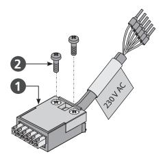
**Note** Locking hooks - at the housing cover **1** - prevent withdrawal of the plug under tensile load.
