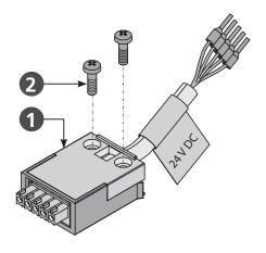
**NOTE** Locking hooks - at the housing cover **1** - prevent withdrawal of the plug under tensile load.
