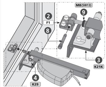
■ Adjust casement pressure - using of the nut M8 (SW13)
